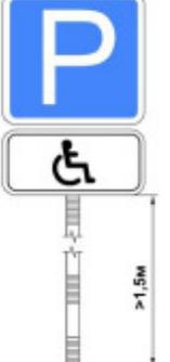
A diagram of a vertical parking sign. It consists of a blue square sign with a white 'P' and a white wheelchair symbol below it. The sign is mounted on a vertical post. A dimension line to the right of the post indicates a height of >1.5m.                                                                                     | Знаков нет | Привести в соответствие |
